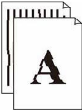
Lines Are Misaligned/Distorted
