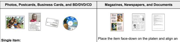
Place the item face-down on the platen, with 0.4 inch (1 cm) or more space between the edges (diagonally striped area) of the platen and the item. Portions placed on the diagonally striped area cannot be scanned.
