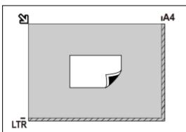
Place the item face-down on the platen and align an upper corner of the item with the corner at the arrow (alignment mark) of the platen. Portions placed on the diagonally striped area cannot be scanned.
