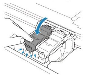
After you install the FINE cartridge, close the scanning unit / cover.
