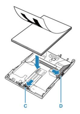
5. Align paper guides (C) in front and (D) on right with paper length and width.
