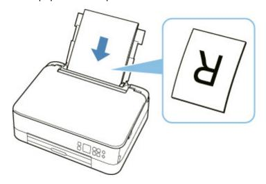
6. Slide right paper guide (D) to align with both sides of paper stack.
