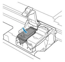
2. Close the ink cartridge locking cover to secure the FINE cartridge.
