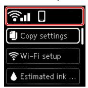
If the icon appears on the LCD, it indicates that Wi-Fi is enabled and the printer is connected to the wireless router.
