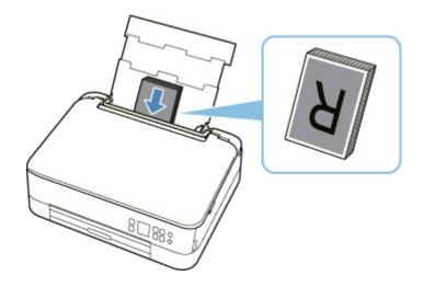
**5.** Slide right paper guide (D) to align with both sides of paper stack.
