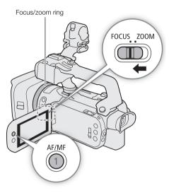
By default, the camcorder will focus automatically on a subject at the center of the screen. If the AF frame size has been changed to an option other than [ $\mathbf{A}$  Automatic] ( $\mathbf{\Box}$  50), the camcorder will focus automatically on a subject inside the AF frame that appears on the screen.
