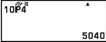
The calculator display shows the result of the permutation function: 10P4 = 5040.
