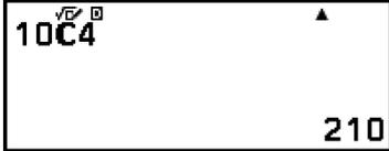
The calculator display shows the result of the combination function: 10C4 = 210.
