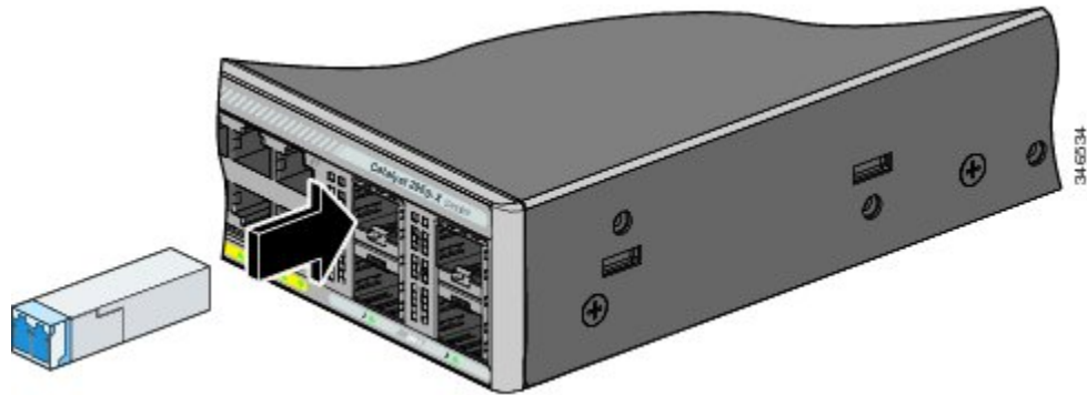
Figure 27: Installing an SFP Module
