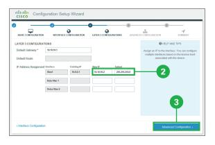
Enter the IP address and subnet mask for the switch in the [New IP] and [Subnet] of [VlanX] row.
