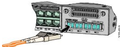
Figure 43: Network Module with SFP Modules Installed
