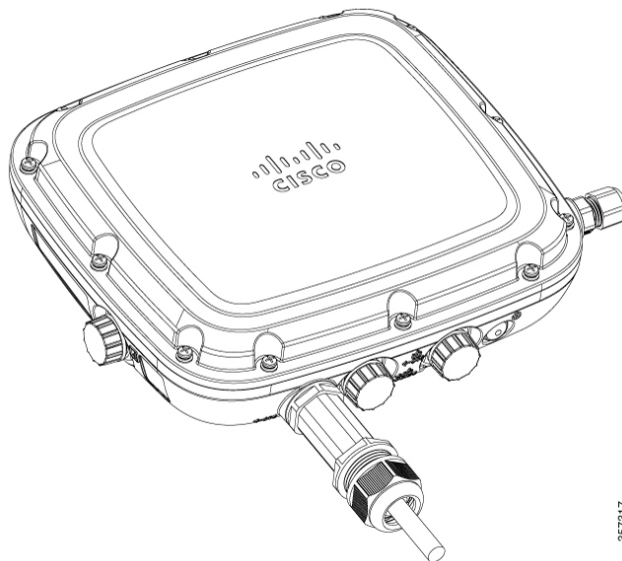
Figure 82: Fiber-Optic cable and gland installed to AP
