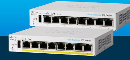
Thank you for choosing the Cisco Business 250 Series Switch. These switches are designed to be operational right out of the box as standard switches. In the default configuration, the switch forwards packets between the connected devices after powering up.
