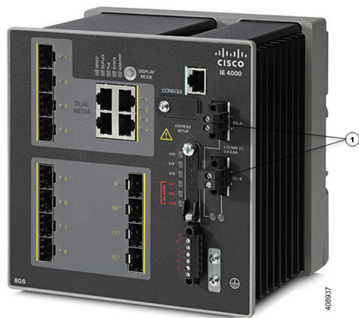
Figure 10 Removing the Power Connectors from the Switch
