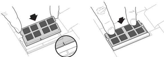
Firmly push the SODIMM in at a 45-degree angle, and then push down until clips snap into place. When it is fully seated in the slot, one-sixteenth of an inch or less of the gold pins will be visible.
