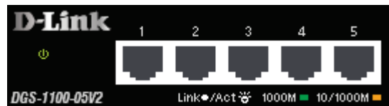
Figure 1.9 –LED Indicators on DGS-1100 series
