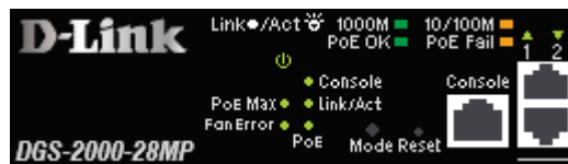
Figure 1.21 –LED Indicators on DGS-2000 series
