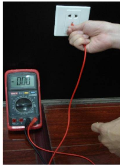
Appendix Figure 7-5 Check earth cable connection
