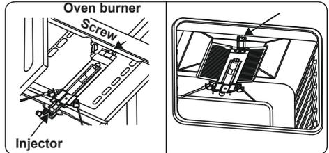
Remove the injectors using a 7mm spanner and replace the injector with the ones from the spare set. Make sure you use corresponding diameters suitable to the type of gas that is going to be used, according to the information chart (which is also supplied in the gas conversion kit).
