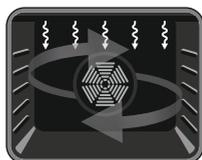
**Grill and Fan Function:** The oven's thermostat and warning lights will switch on, and the grill heating element and fan will start operating. This function is ideal
