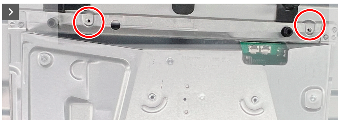
Figure 22. Removing the metal shield
