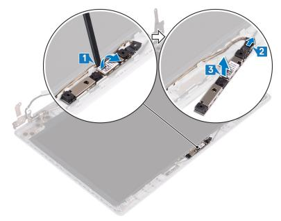
3 Lift the camera module from the display back-cover and antenna assembly.
