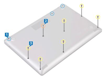
4 Pry the base cover starting from the top-left corner of the computer base.
