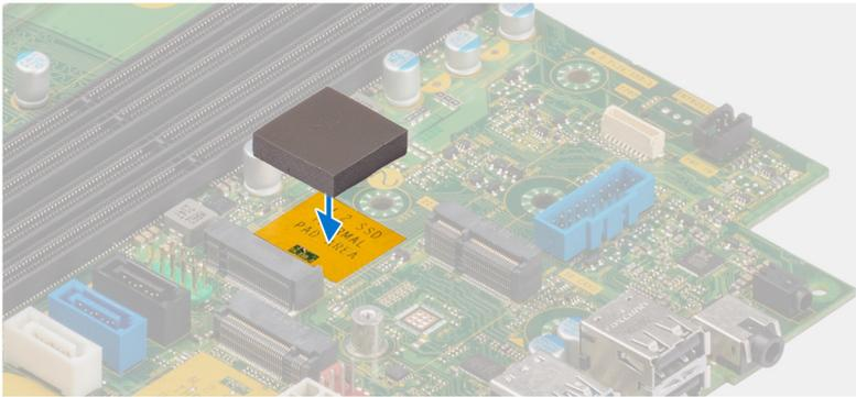
2. Peel off the protection mylar on the thermal pad.
