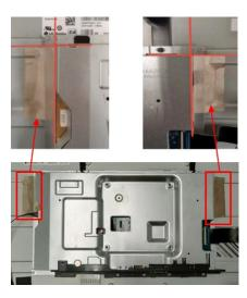
Insert "Backlight wire" to "Panel" and "Power Board"
