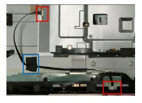
S10 Assemble "USB board" with "USB Shielding"
