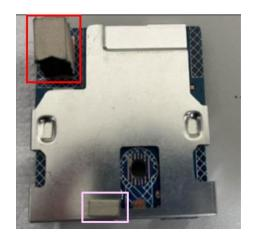
S10 Disassemble "USB board" from "USB Shielding"
