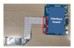
Assemble "Interface board" to "Main Shielding"
