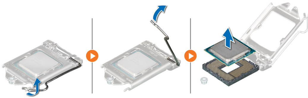
Figure 44. Removing the processor
