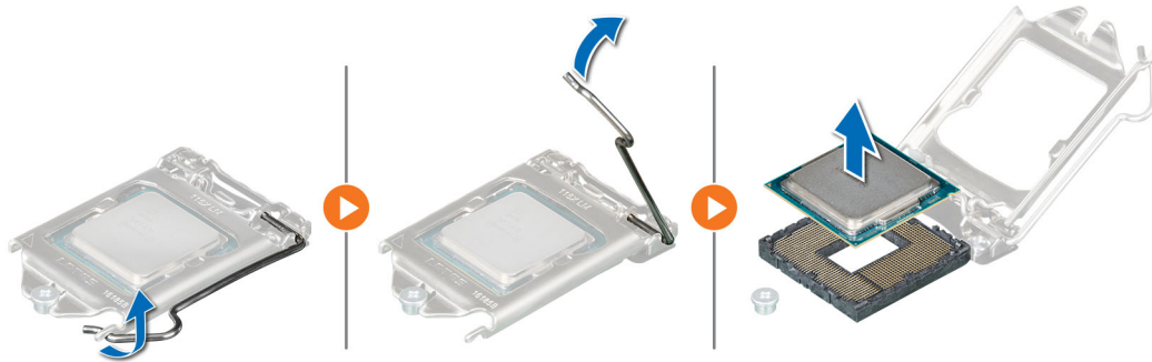
Figure 59. Removing the processor
