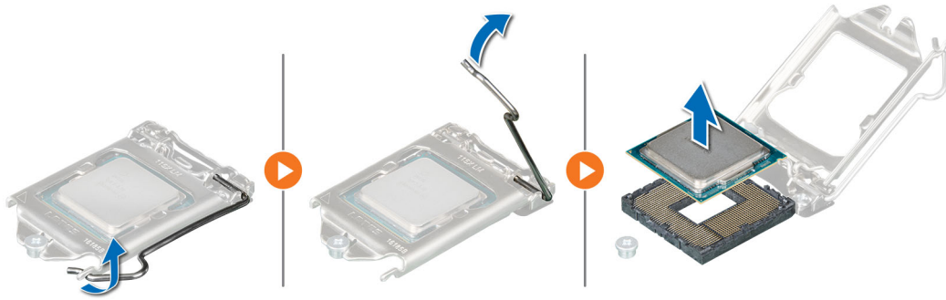
Figure 59. Removing the processor
