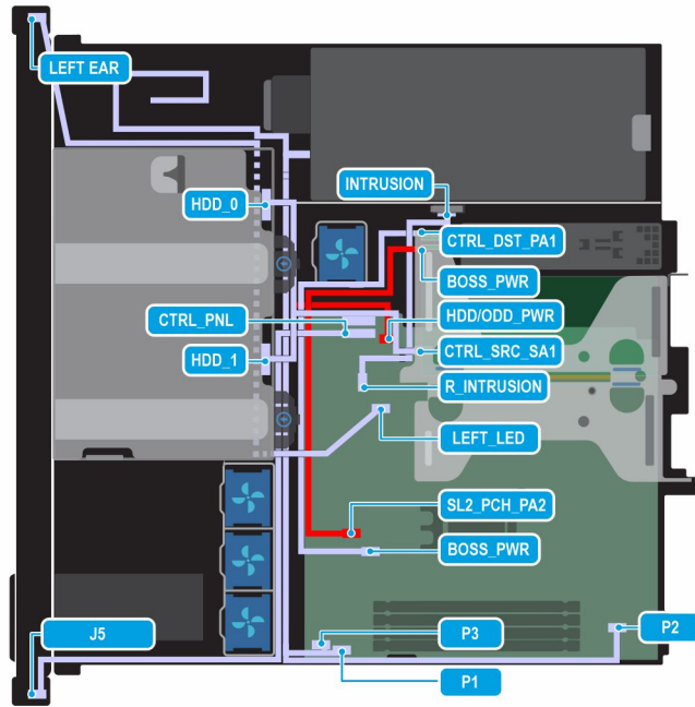
Figure 41. Configuration 2: 2 x 3.5 inch PERC SAS/SATA- no Backplane with cable PSU and BOSS-N1 (optional)
