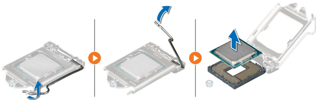
Figure 43. Removing the processor
