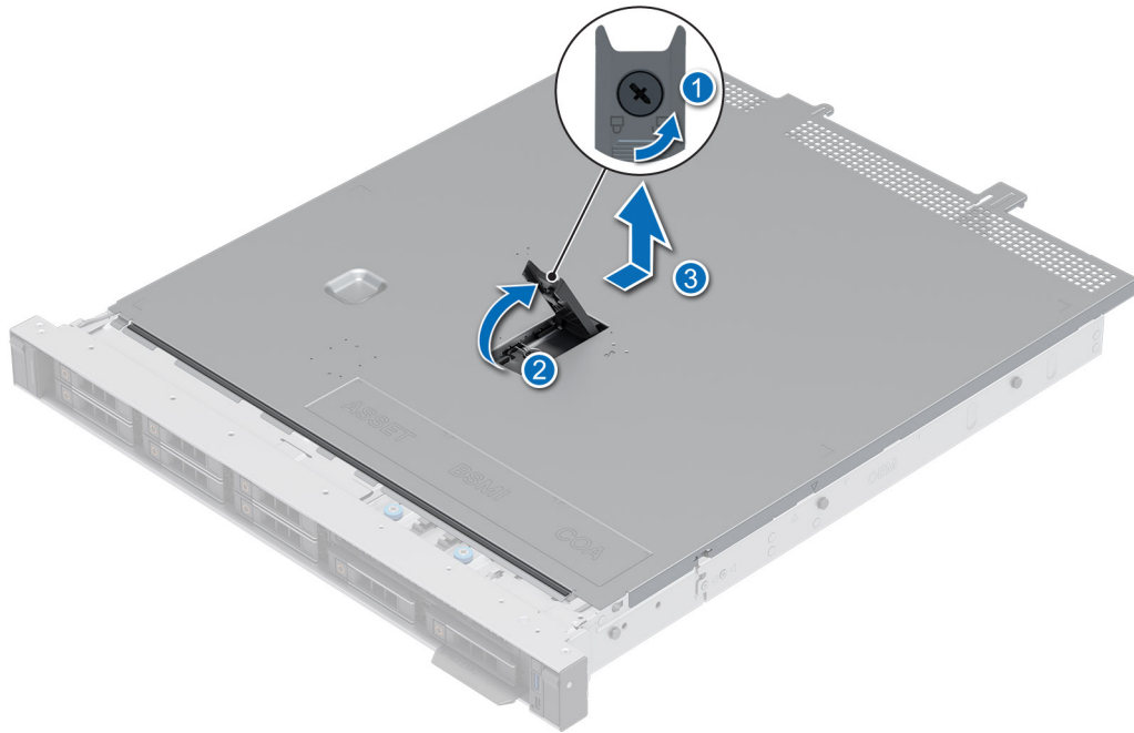
Figure 11. Removing the system cover
