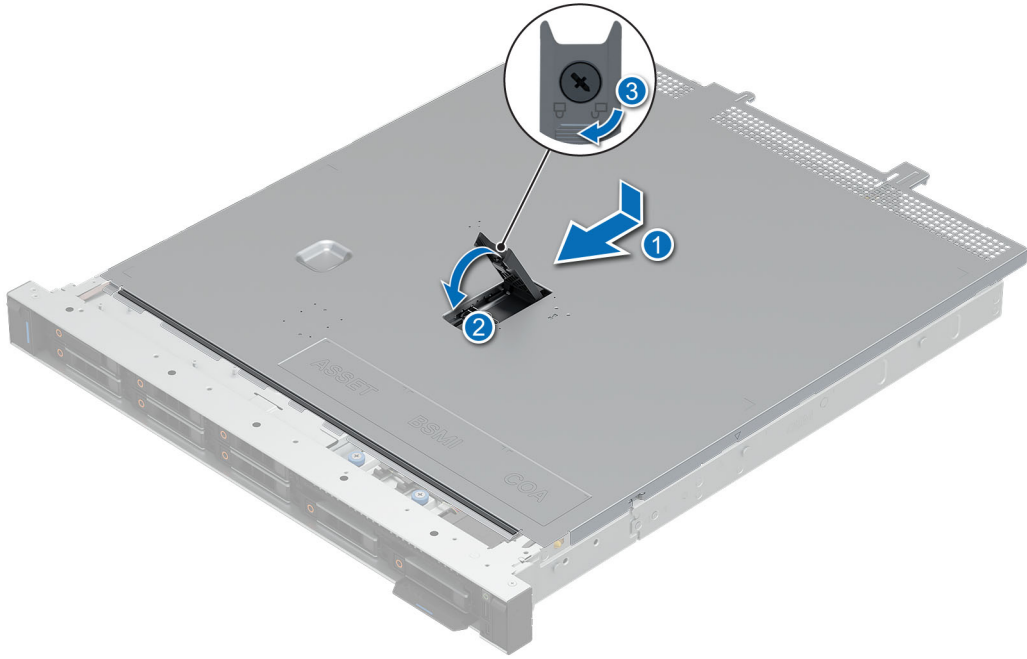
Figure 17. Installing system cover
