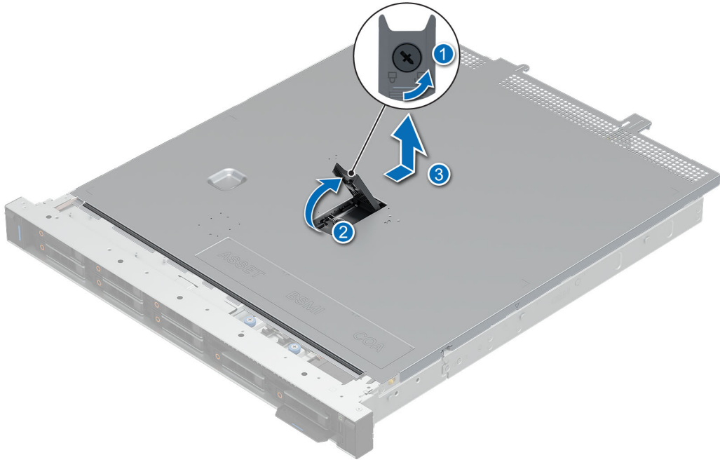
Figure 16. Removing the system cover
