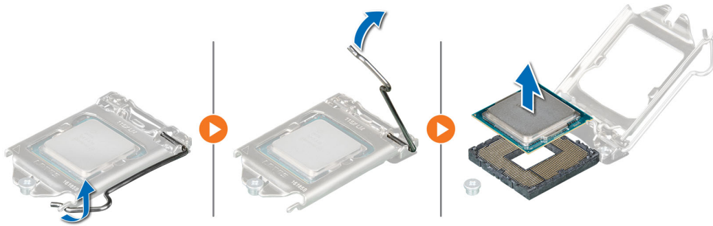
Figure 45. Removing the processor
