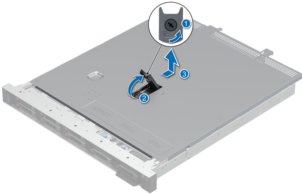
Figure 16. Removing the system cover
