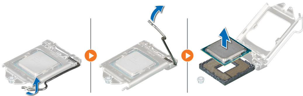
Figure 45. Removing the processor
