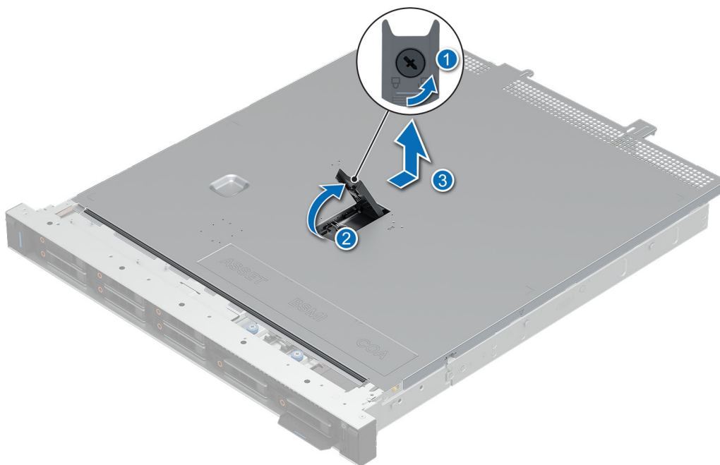
Figure 16. Removing the system cover
