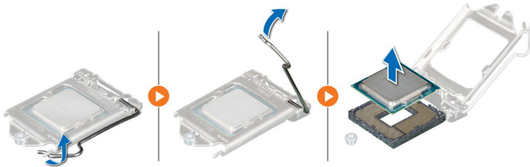
Figure 45. Removing the processor
