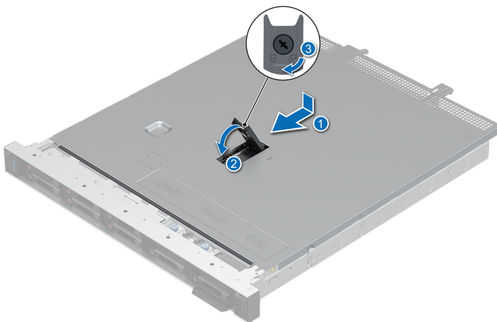
Figure 17. Installing system cover
