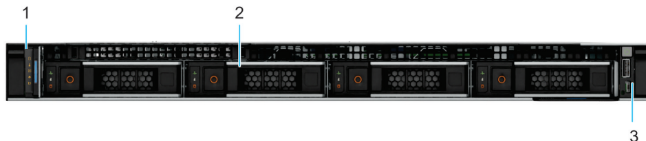
Figure 1. Front view of 4 x 3.5-inch drive system
