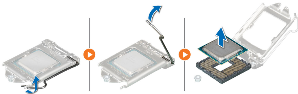
Figure 45. Removing the processor
