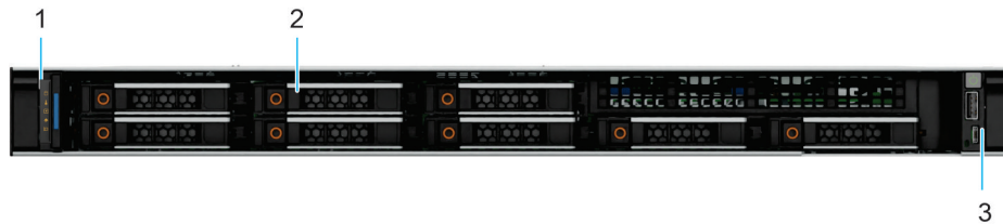
Figure 2. Front view of 8 x 2.5-inch drive system
