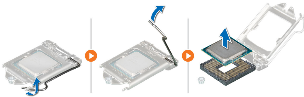
Figure 45. Removing the processor
