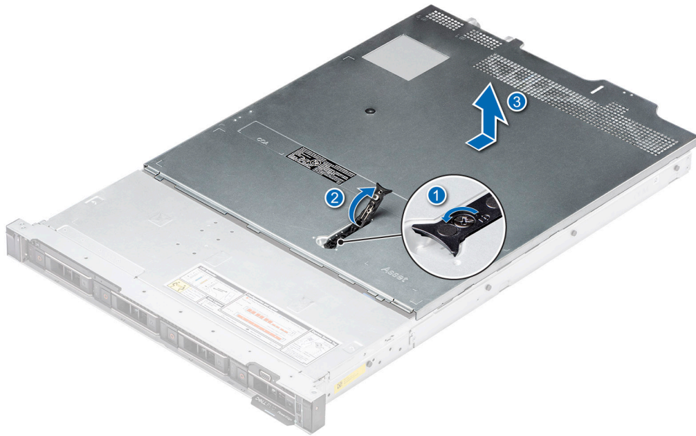
Figure 17. Removing the system cover
