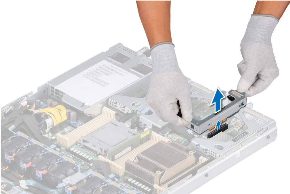
Figure 76. Removing the M.2 BOSS riser
