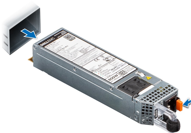
Figure 96. Removing a power supply unit
