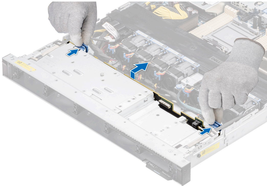
Figure 37. Removing the backplane
