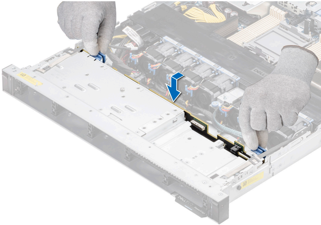
Figure 38. Installing the drive backplane
