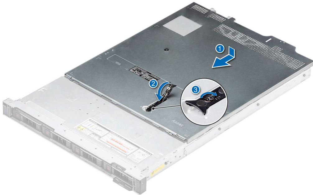
Figure 18. Installing the system cover
