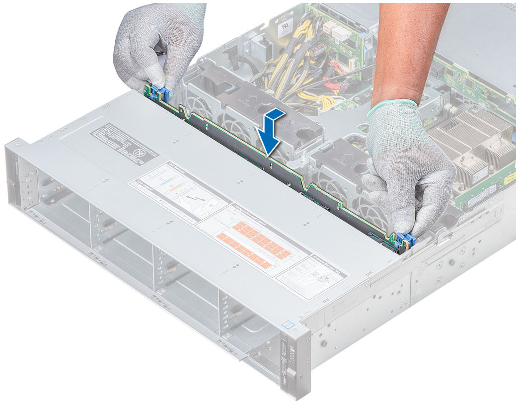
Figure 101. Installing the backplane
