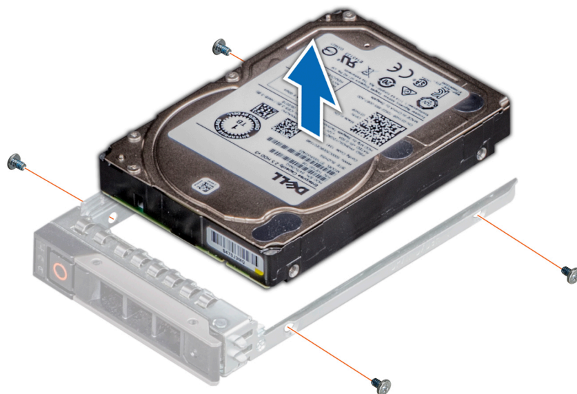
Figure 52. Removing the drive from the drive carrier
