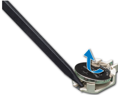
Figure 111. Removing the system battery
