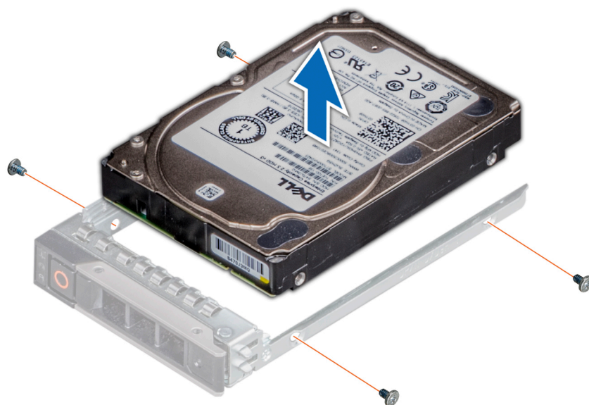
Figure 53. Removing the drive from the drive carrier
