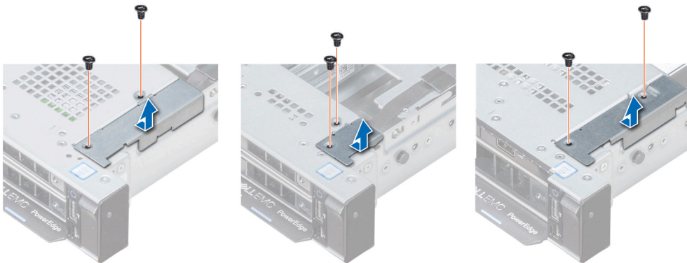
Figure 123. Removing the cable cover
