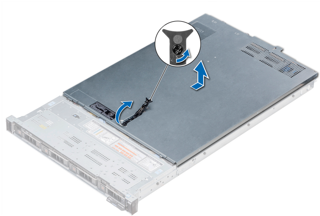
Figure 21. Removing the system cover
