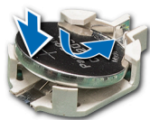
Figure 105. Installing the system battery
