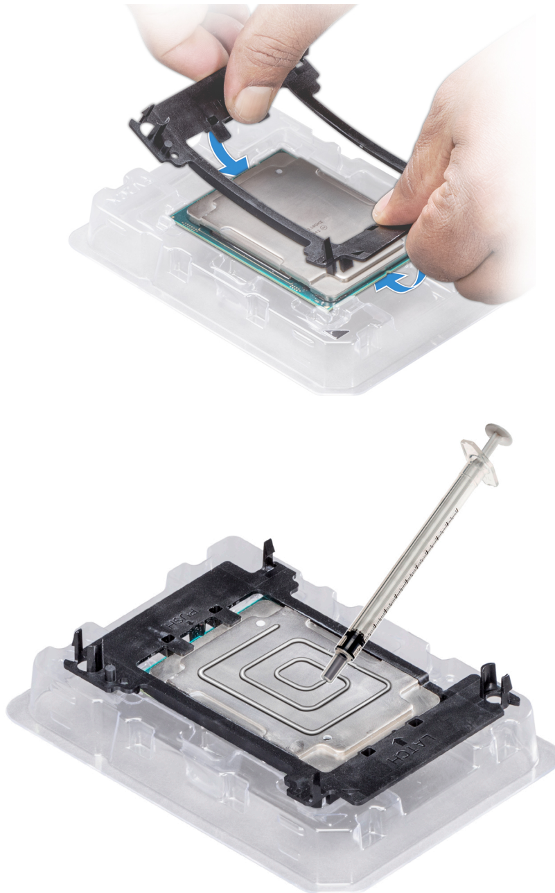
Figure 47. Applying thermal grease on top of the processor
