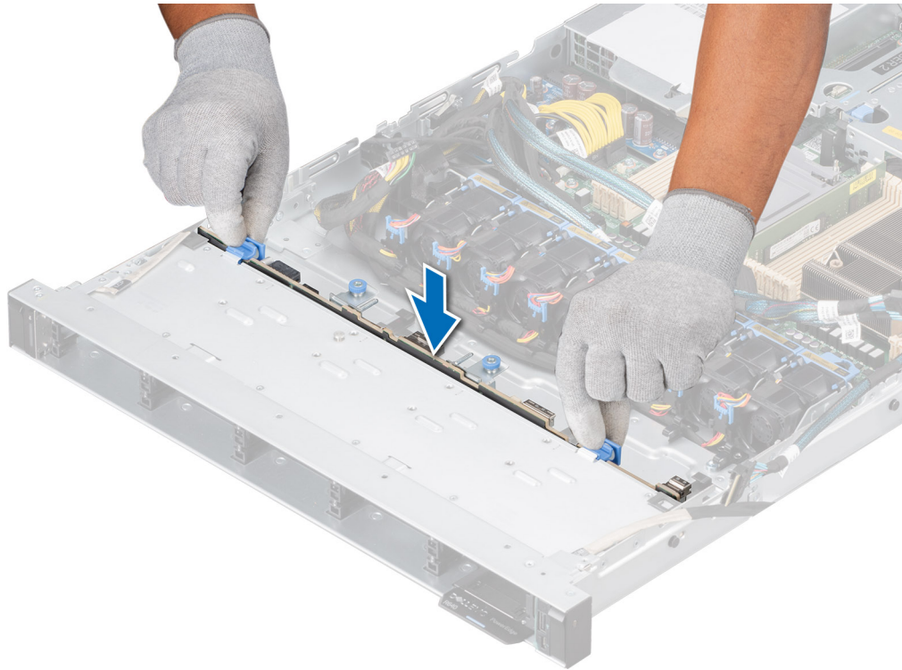
Figure 36. Installing the drive backplane
