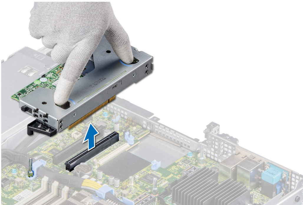
Figure 54. Removing the low profile left riser
