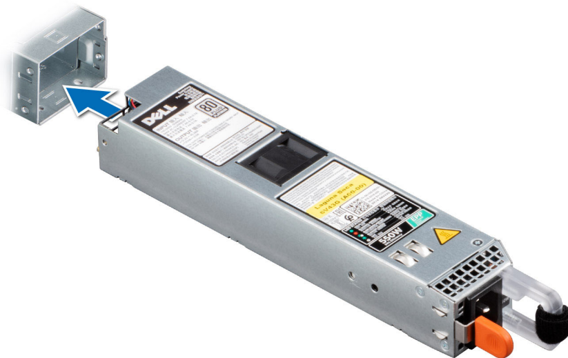
Figure 92. Installing a power supply unit
