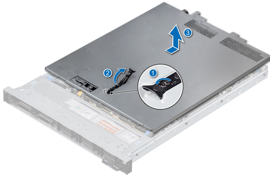
Figure 17. Removing the system cover
