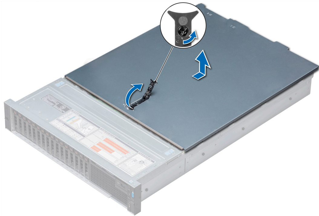
Figure 25. Removing the system cover
