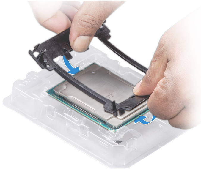
Figure 60. Installing the processor bracket
