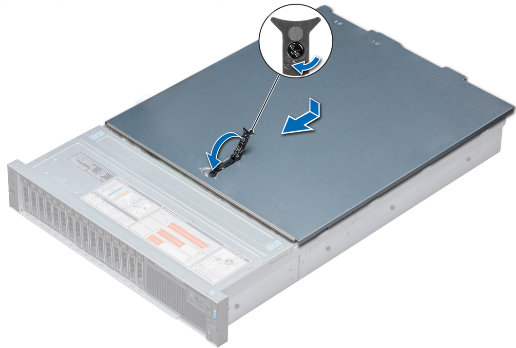
Figure 26. Installing system cover
