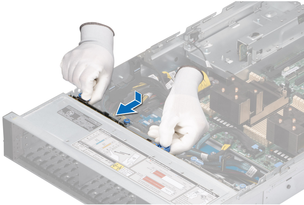
Figure 50. Installing the drive backplane
