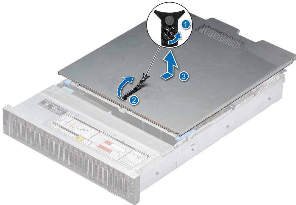
Figure 19. Removing the system cover
