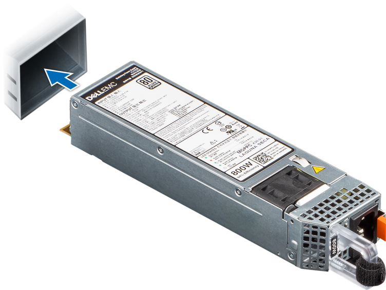
Figure 129. Installing a power supply unit
