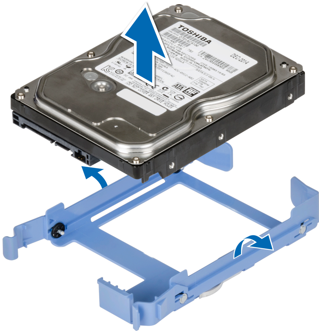
Figure 14. Removing the drive from the drive carrier
