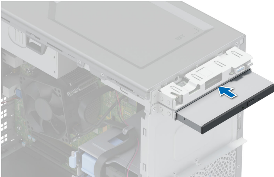
Figure 27. Installing the optical drive
