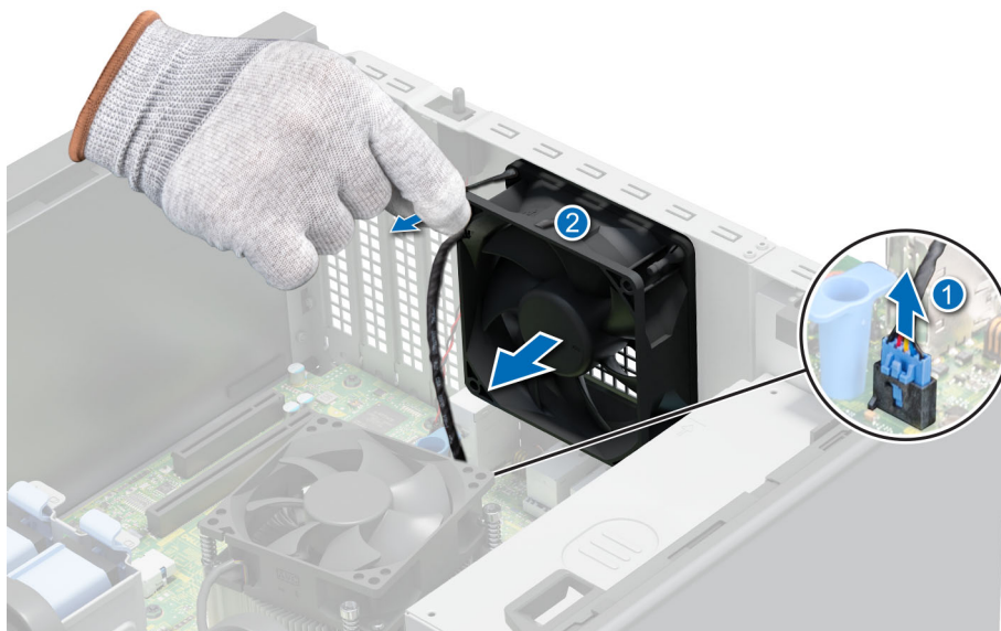
Figure 32. Removing the cooling fan
