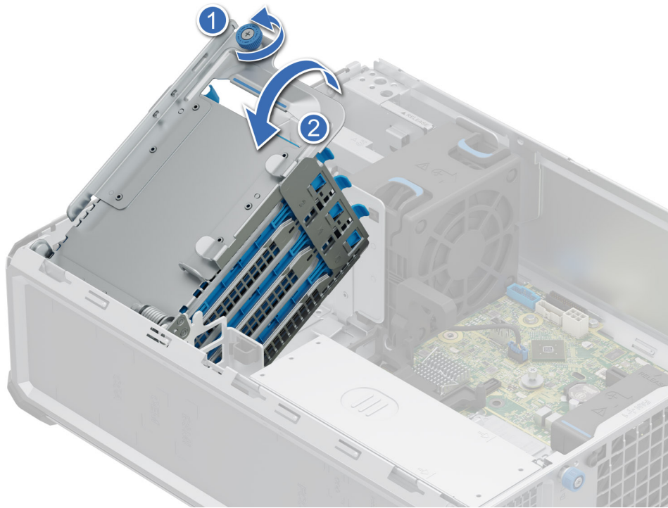
Figure 18. Removing a drive from drive cage
