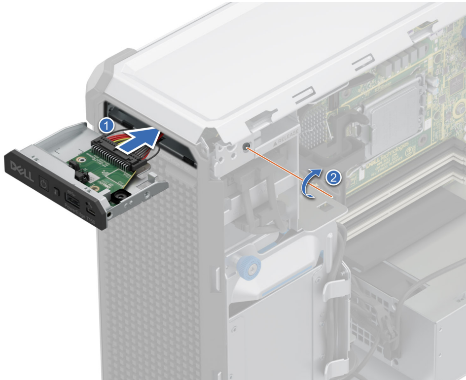
Figure 69. Installing the control panel cage
