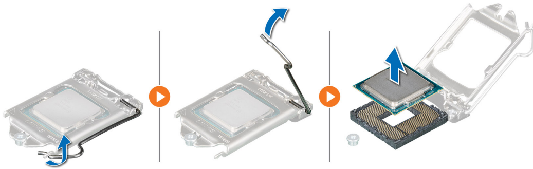
Figure 38. Removing the processor
