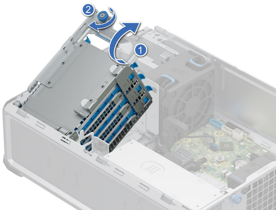
Figure 22. Installing a drive carrier
