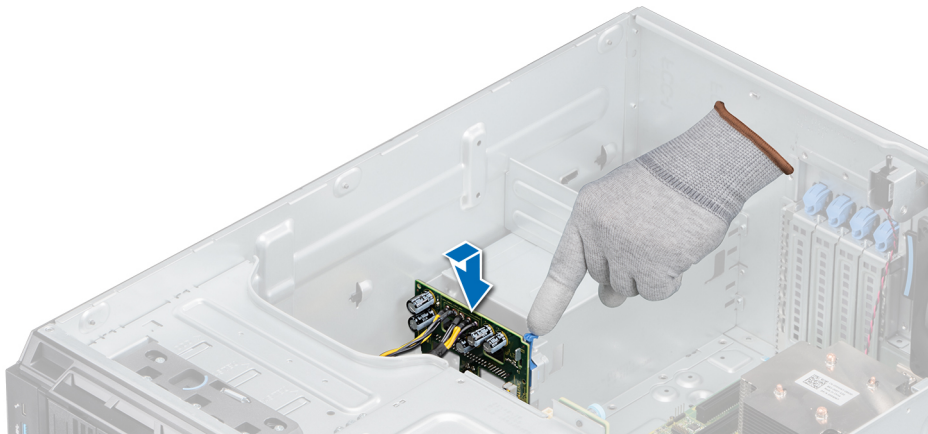
Figure 77. Installing the power interposer board
