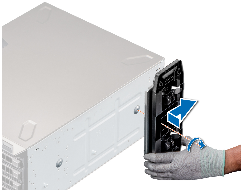
Figure 21. Installing caster wheels
