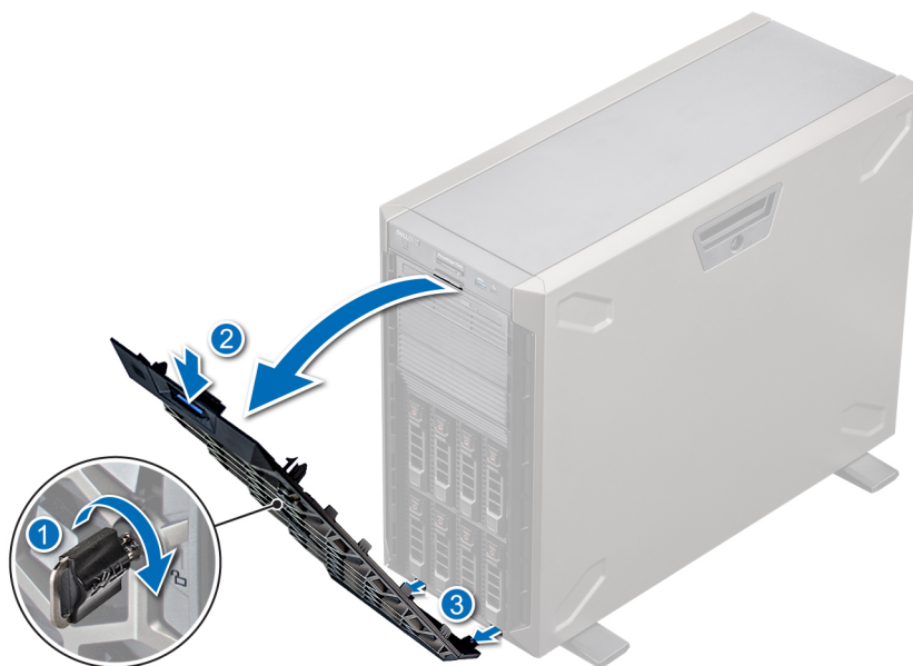
Figure 17. Removing the front bezel
