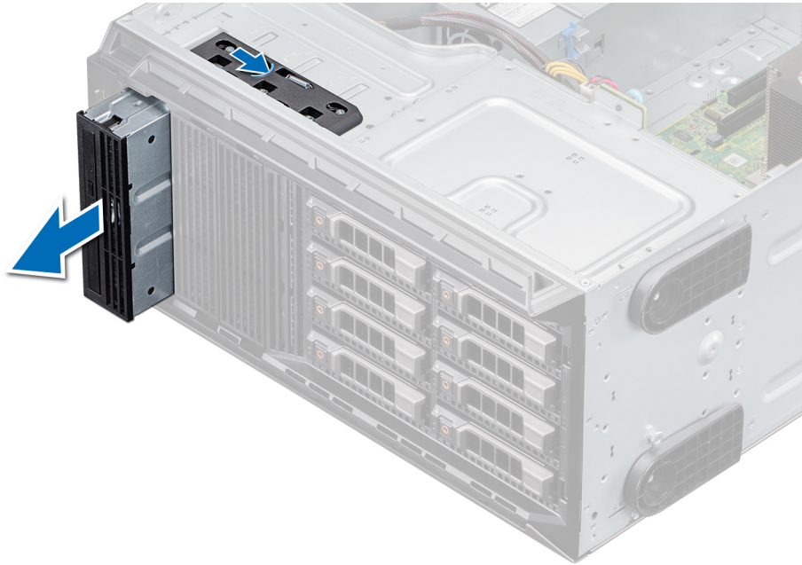
Figure 40. Removing the optical drive
