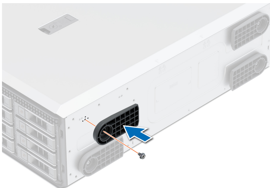
Figure 15. Installing the system feet
