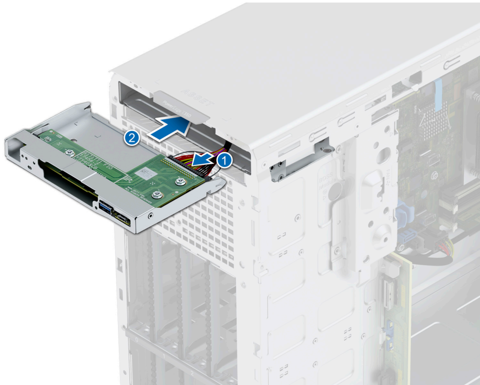
Figure 99. Installing the control panel cage
