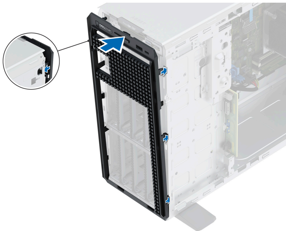
Figure 100. Installing the front faceplate
