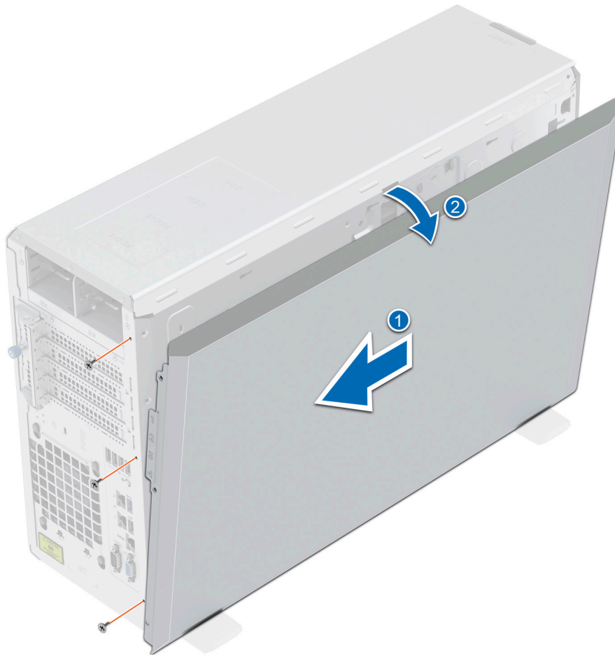
Figure 94. Removing the system side cover
