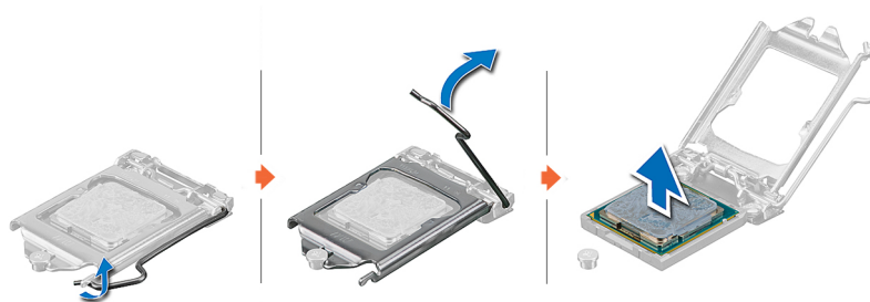
Figure 50. Removing the processor
