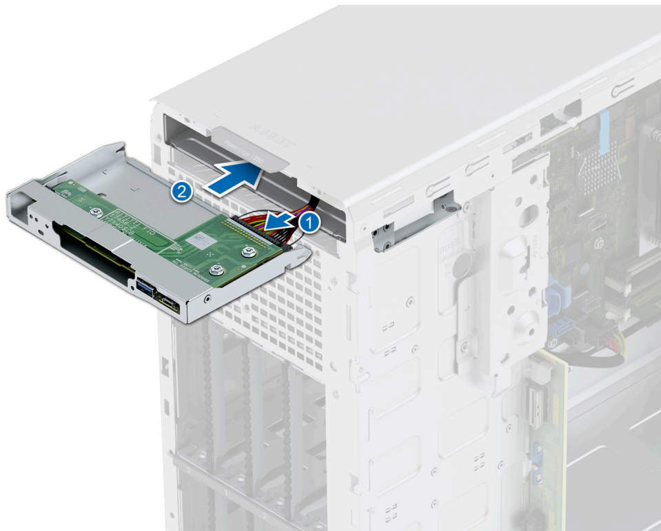
Figure 99. Installing the control panel cage
