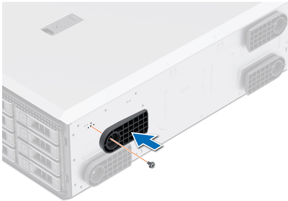
Figure 15. Installing the system feet
