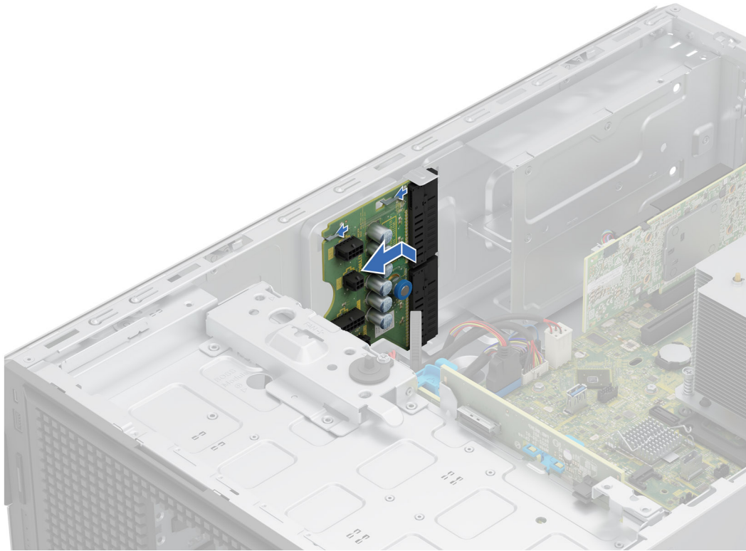
Figure 85. Installing the power interposer board
